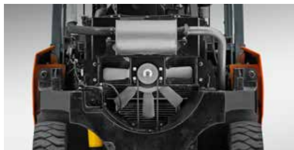
The fan, radiator, integrated torque convertor cooler and hydraulic oil cooler prevent engine overheating. Thus, performance is kept to a maximum.
